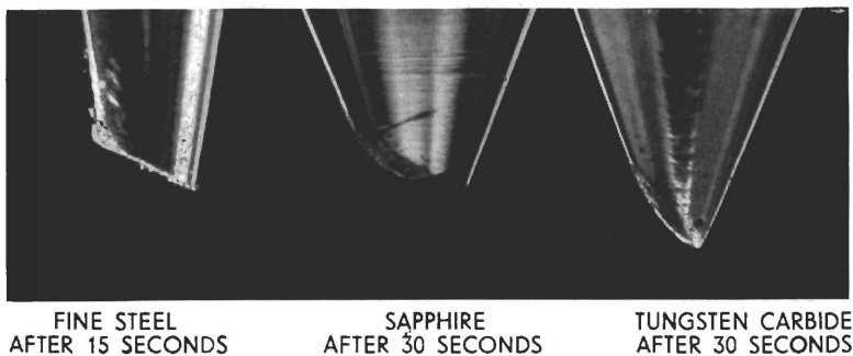
FIG. 62/4.—Abrasive tests on needle points.
