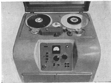
FIG. 49—E.M.I. Tape Recorder. View of tape driving mechanism, head assembly and control panel.
