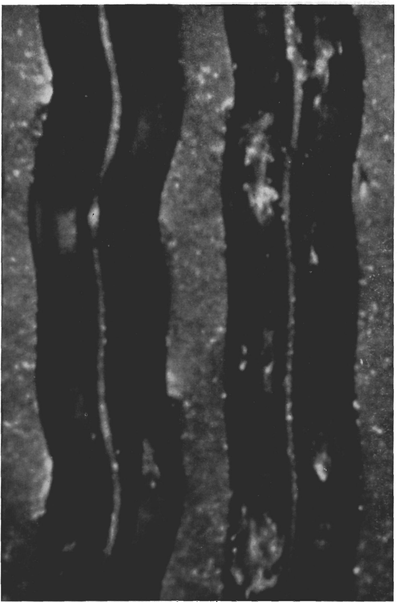
MODERN SHELLAC DISC AFTER ONE PLAYING WITH STEEL NEEDLE Photo by C. E. WATTS. 200X.
