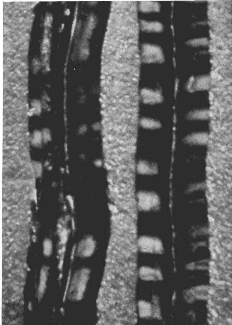
0.005" MODERN SHELLAC DISC AFTER TWENTY PLAYINGS WITH SAPPHIRE IN ORDINARY LIGHT-WEIGHT PICKUP
